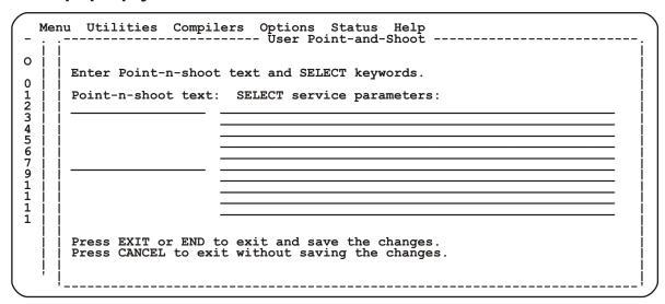
Place text in the first column and ISPF service requests in the second column; on display, the text shows in the status area and clicking on the text invokes the ISPF service
